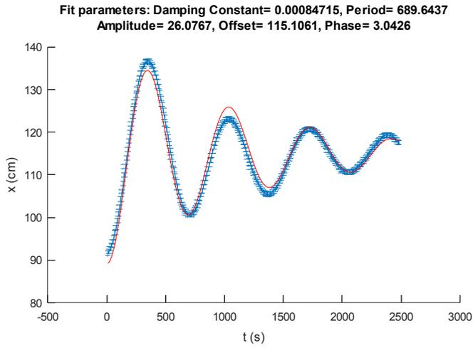
FIG. 4. Fit curve to the data that we collected by moving the large masses from position 1 to position 2. The error in the data points is  $\alpha_x = 0.05\text{cm}$ . The values of the fit parameters of equation (12) are reported above the plot. In this case, the value of the offset is equal to  $x_{\text{eq}}$ .
