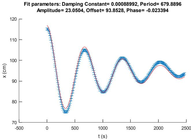
FIG. 3. Fit curve to the data that we collected by moving the large masses from position 2 to position 1. The error in the data points is  $\alpha_x = 0.05\text{cm}$ . The values of the fit parameters of equation (12) are reported above the plot. In this case, the value of the offset is equal to  $-x_{\text{eq}}$ .
