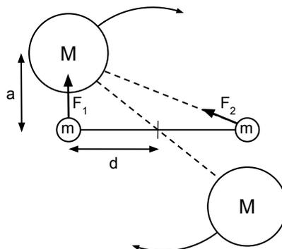
FIG. 1. This is a schematic diagram of the top-down view of the torsion pendulum with two small masses  $m$  and larger masses  $M$  set in one of the two positions.
