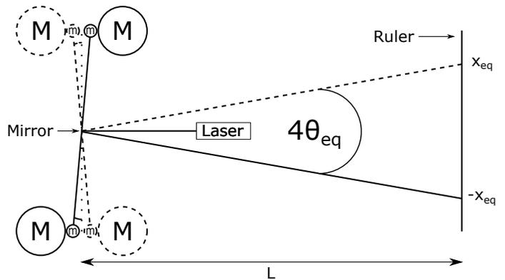
FIG. 2. Above view of our apparatus. The solid line shows the apparatus in position 1, while the dashed line shows the apparatus in position 2. When the apparatus is in position 1, the barbell is at  $-\theta_{\text{eq}}$  and the laser is at  $-x_{\text{eq}}$ . When the apparatus is in position 2, the barbell is at  $\theta_{\text{eq}}$  and the laser is at  $x_{\text{eq}}$ .
